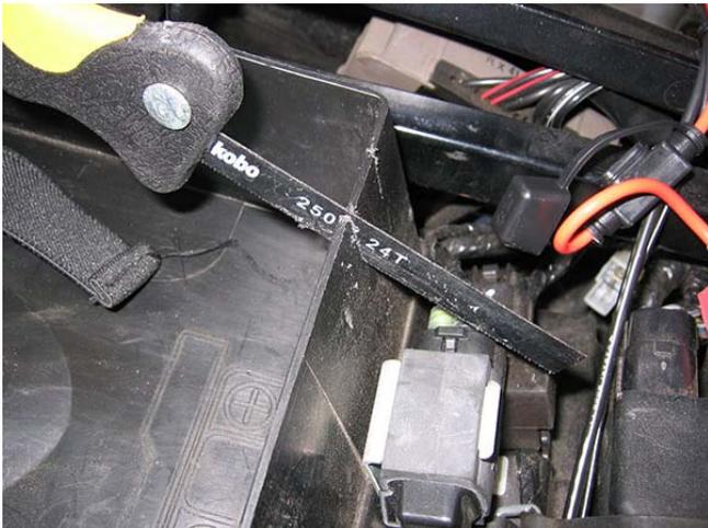
To the left you can see how I cut two slots for the wire entrance. Bending the cutout into a little ramp made a nice place to cable tie my wires.
